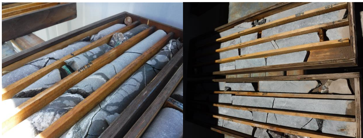
Figure 12.1. Whole and Split core from Pacific Copper’s 2008-2009 drill program.
