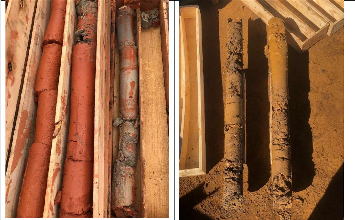
Figure 27: Examples of core obtained using Sonic drilling (Hill 2022)
