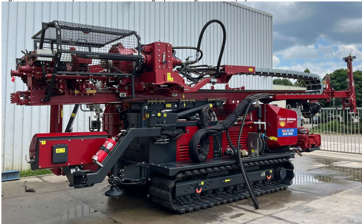
Figure 26: Photograph of the sonic rig to be used at the Madeira Project (Scervini 2023)
