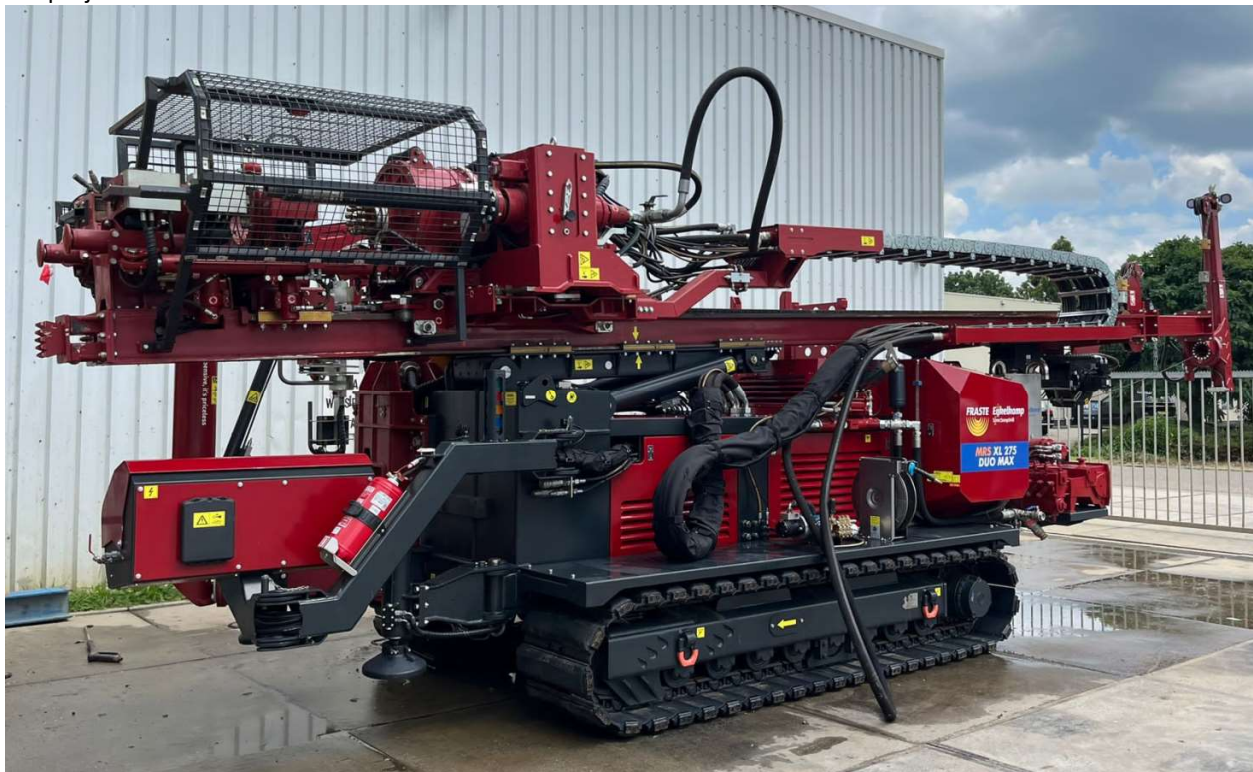
Figure 28: Photograph of the sonic rig to be used at the Madeira project
