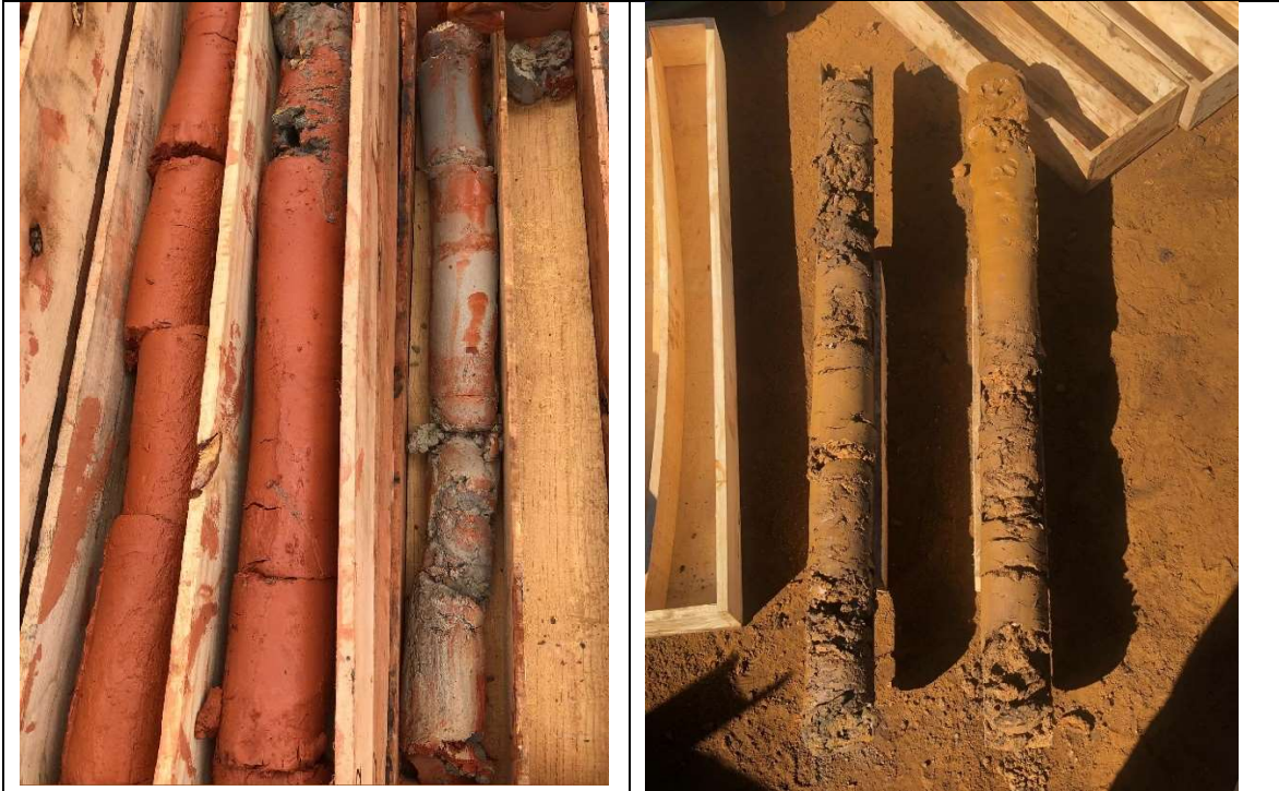
Figure 29: Examples of core obtained using Sonic drilling
