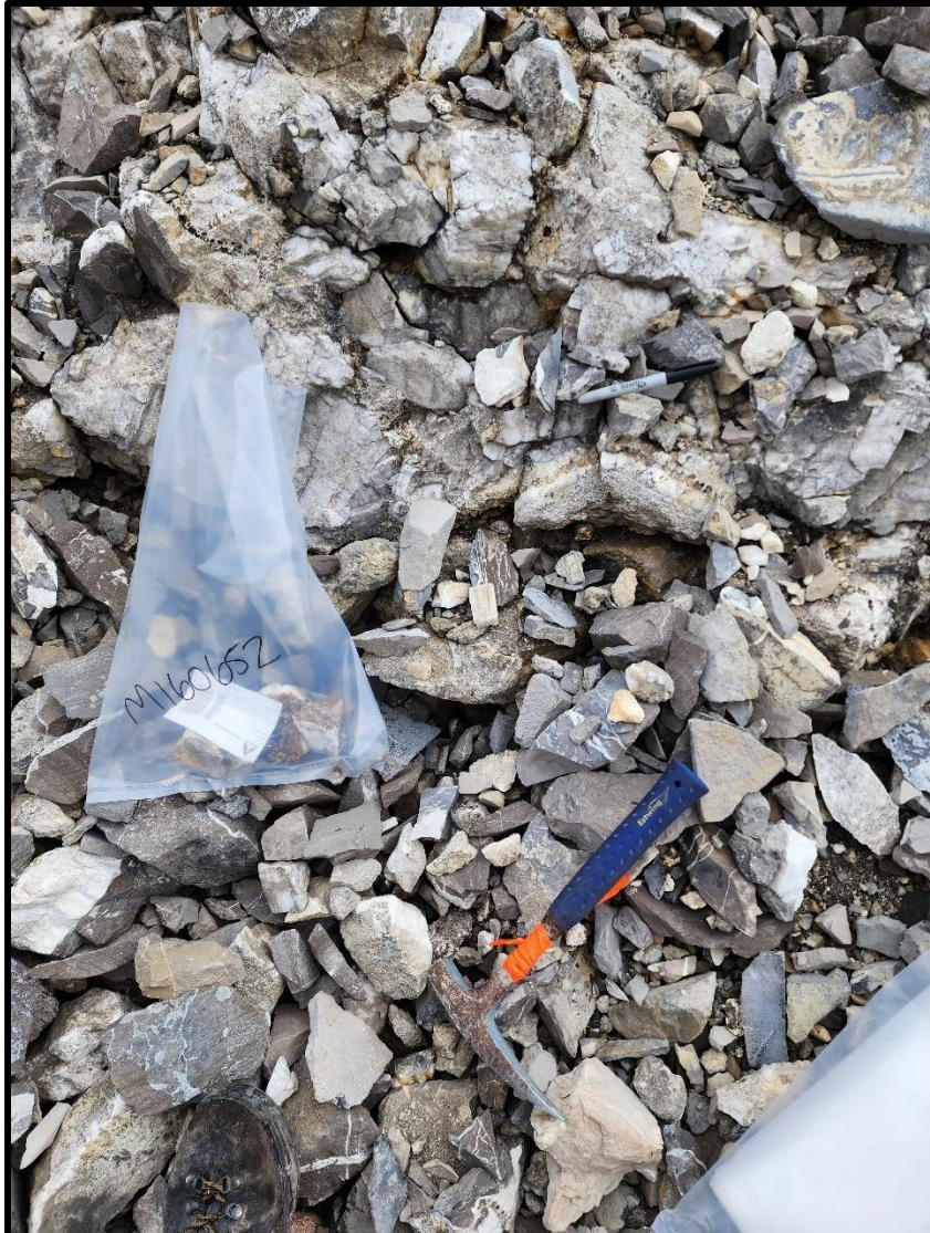
Figure 14 Photo example of a rock hand sample being collected, tagged and stored by the author for geochemical analysis during the 2024 exploration program.
