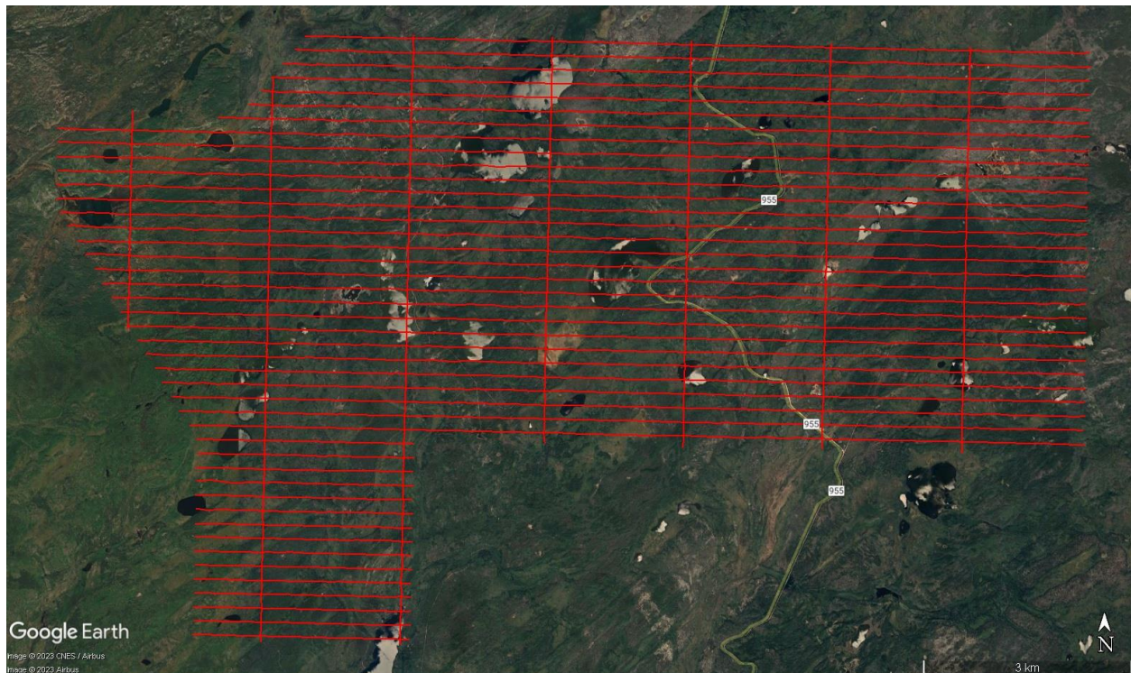
Figure 11 Gorilla Lake Heli-TEM Flight Lines
