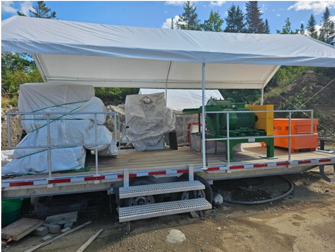
Figure 2: Mobile crusher equipment for use in pilot plant facility
