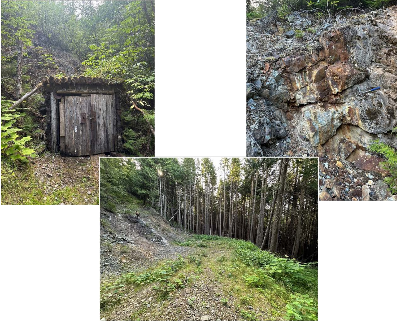
Figure 16 Site visit photographs: Historical portal to Dardanelle Adit (above); Dardanelle showing with steep dipping quartz-sulfide vein in hangingwall to rhyolite dyke and footwall to sheared granodiorite (top right); Location of 2021 drilling (bottom middle)
