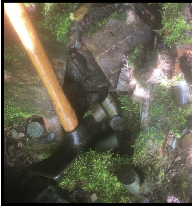
Photo 2-1 Core from an early drill program found to be disturbed (hammer for scale)
