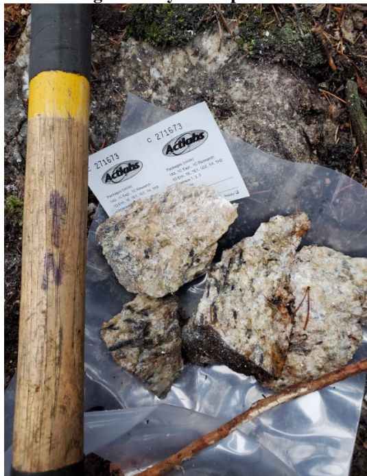
Photo 2: Pegmatite dyke sample C271673. Assay 9.5 ppm Cs and 242 ppm Rb.
