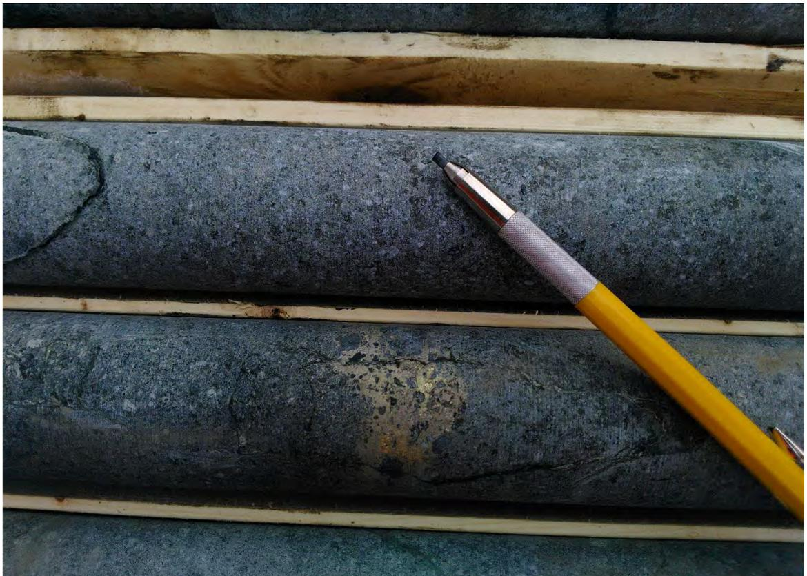
Figure 38. Po + Cp sulphide aggregate
