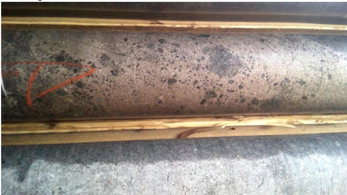
Figure 36. 12 cm of massive Po with olivine inclusions
