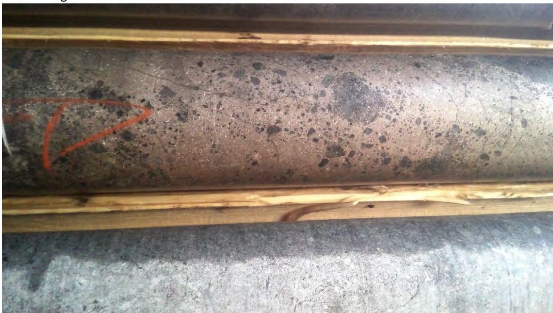
Figure 36. 12 cm of massive Po with olivine inclusions
