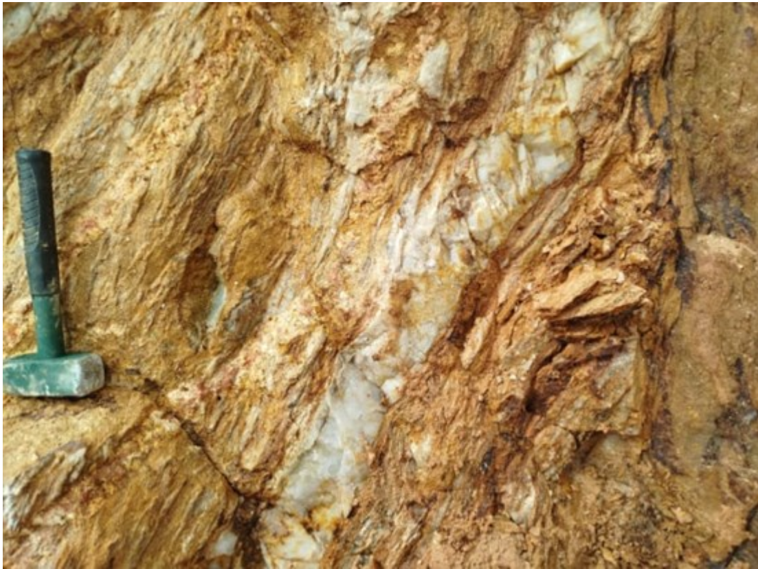
Figure 2. High-grade quartz veins in the Stranger Pit. Sampling of this occurrence yielded 133.25 g/t Au.
