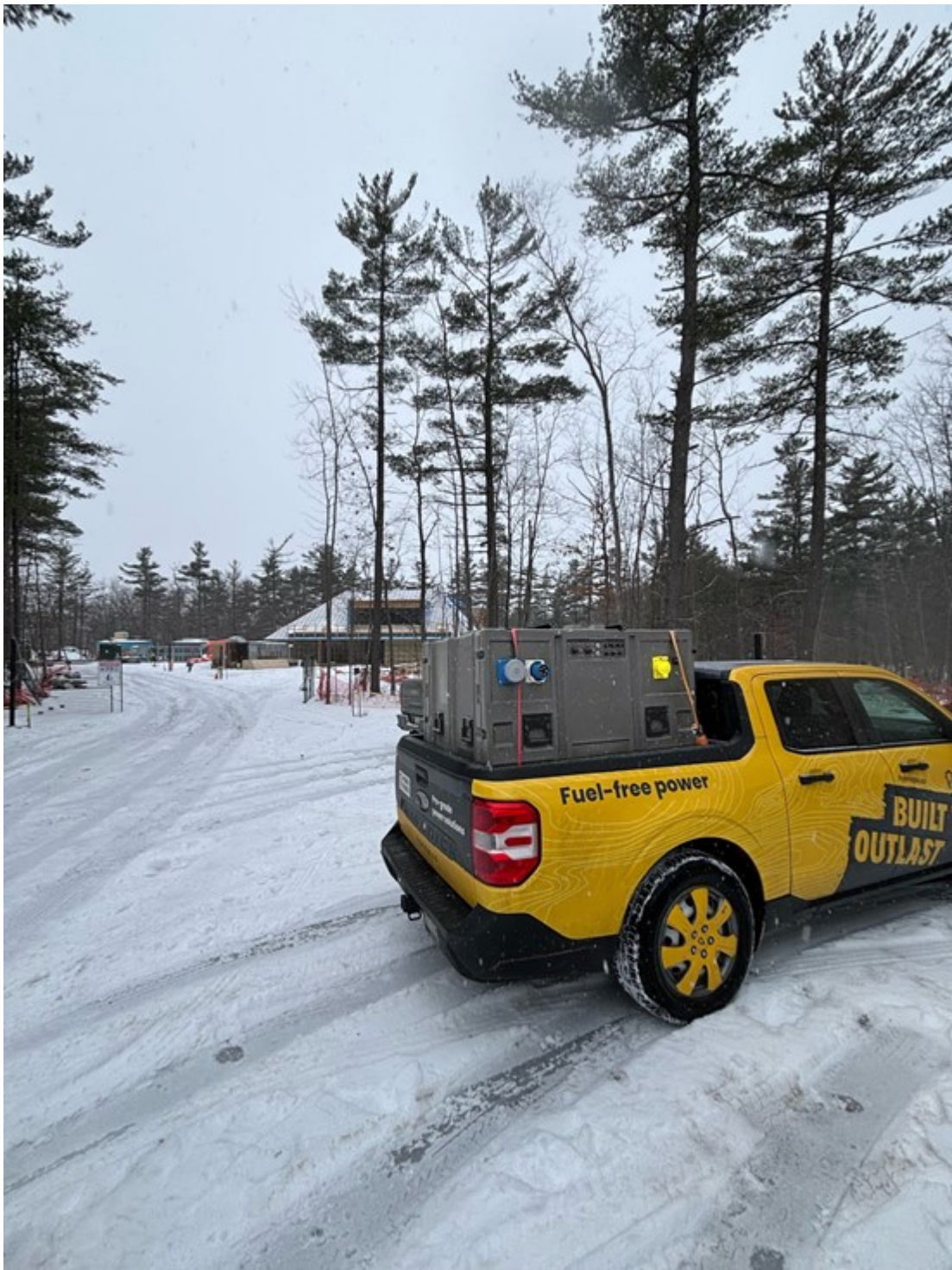
Figure 2: Batt Pack Spark unit mounted on a standard pickup truck bed
