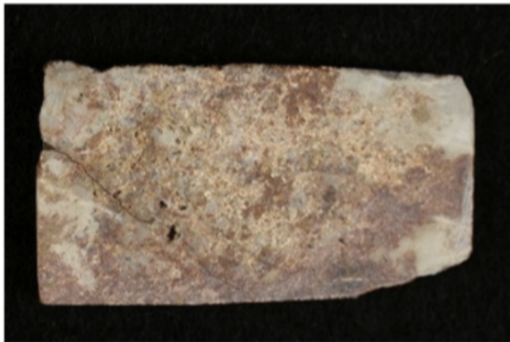
Figure 12. REE mineral-rich cumulate within carbonatite from the CIM drilling (Dalsin, 2011; Dalsin and Groat, 2012).
