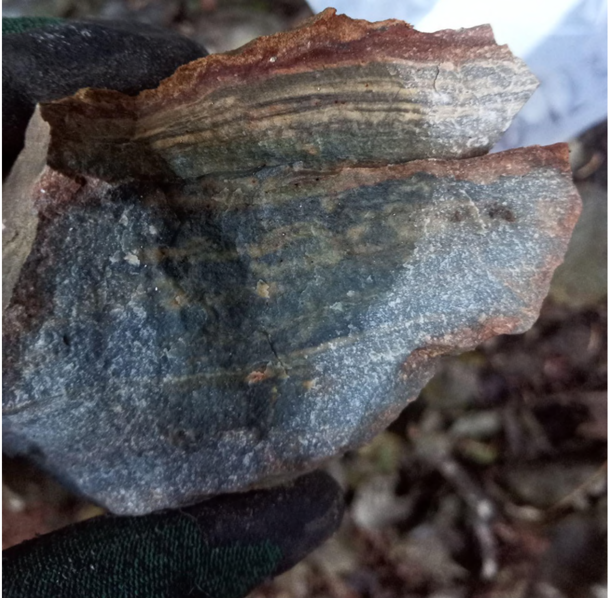
Figure 22 showing rock 69233 returned over-limit results that are today being re-assayed. It shows finely bedded limestone with beds of secondary biotite. Calcite veins up to 1 mm and 10% of rock. 3% fine-grained disseminated iron oxide alteration. Pervasive fine-grained biotite through layers. Minor chlorite alteration. Float likely localized. Found on top of an outcrop under tree, exposed over 10m.
