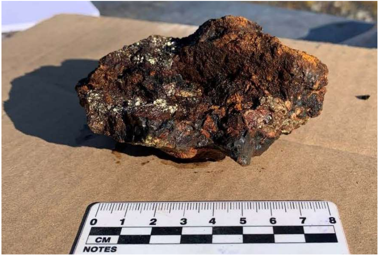
Figure 4: Oxidized Shear Sample EMFIR015 at the Inferno Zone (1.88% Cu, 4.68 g/t Au, and 76.50 g/t Ag).
