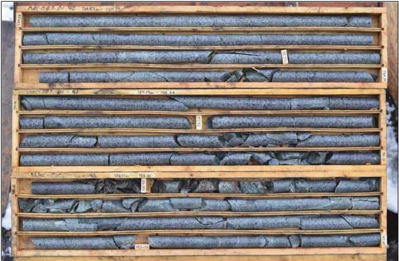
FIGURE 11-1. EXAMPLE OF PHOTOGRAPHED CORE FROM DRILL HOLE MRC-007, BOXES 40 TO 41 (SHANNON BAIRD, 2022).
