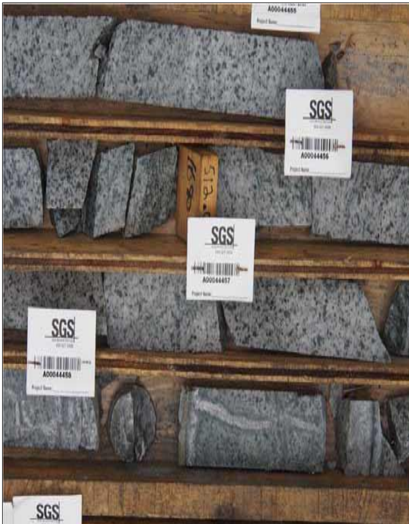
FIGURE 6-8. STOCKWORK-BOXWORK VEINING AT THE END OF DRILL HOLE MRC-006 (GARCIA, 2012B).
