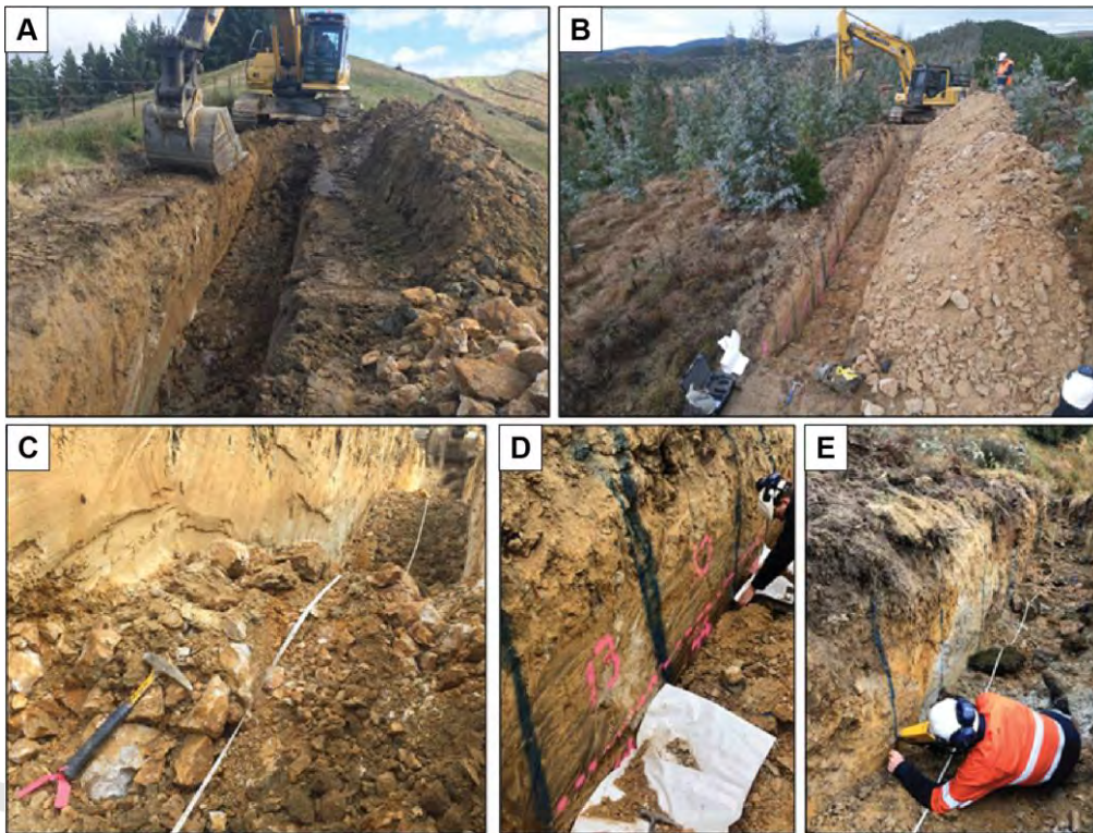
Figure 9-5: Photographs from the trenching campaigns. A) Trench 12 before mark-up; B) Trench 13 after mark-up; C) quartz vein outcrop in Trench 02; D) close-up photograph of the trench mark-up with the tarpaulins laid to collect the sample; E) pXRF analysis of one of the trenches.
