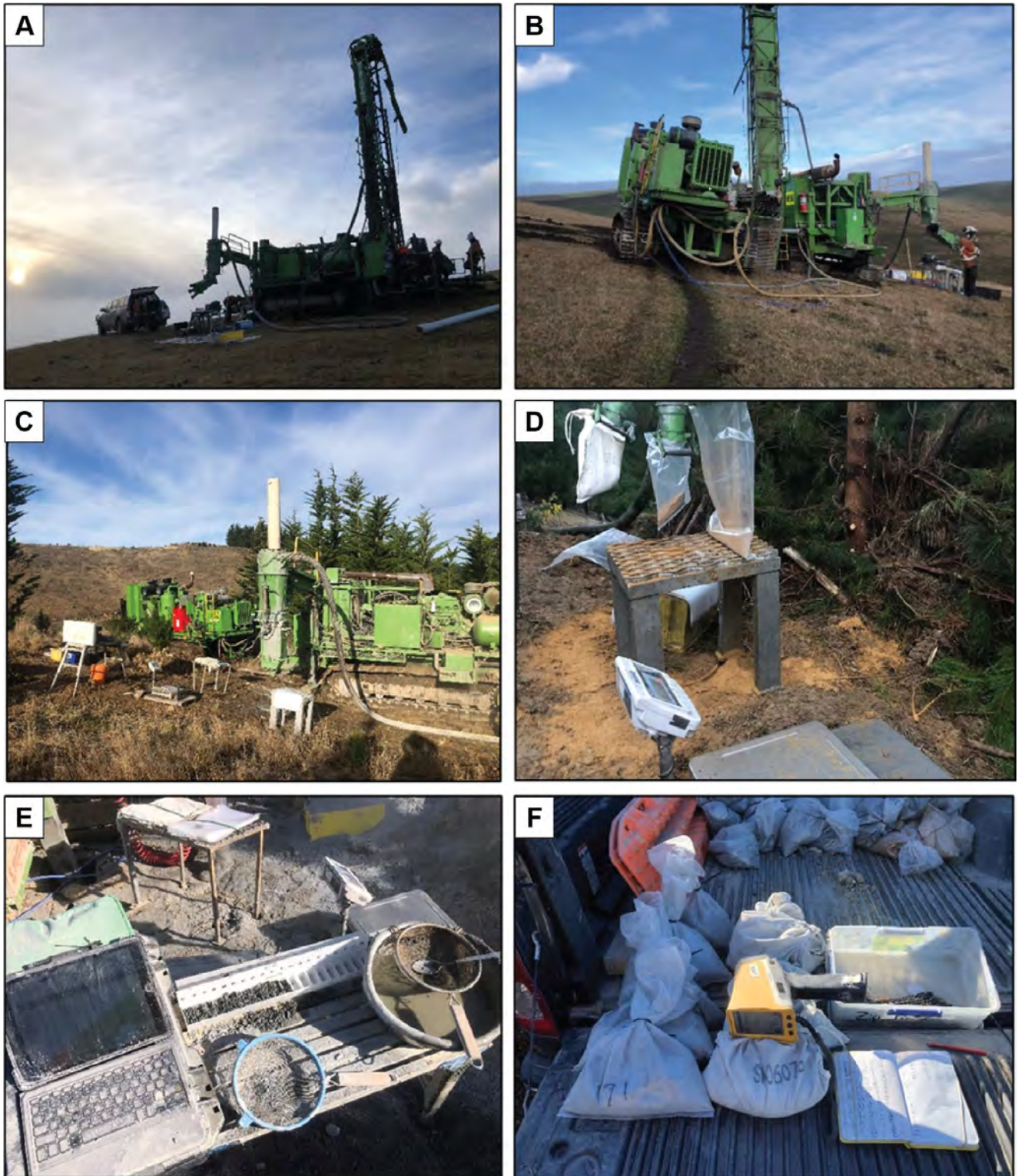
Figure 10-6: A) Photography of the Schramm T660 H Rotadrill drill rig mounted on a CAT325 wide track unit with a Sullair 900cfm x 350 psi air compressor. B) Komatsu CD1 crawler unit with an additional M41 1800 cfm x 870 psi booster assisting the rig. C) View of the sample set-up and rig with a three-tier splitter. D) Splits A, B and C attached to the splitter with scales nearby for weighing samples. E) Logging set up with iPad for recording entered data and chip trays, with wet sieved RC chips. F) Split A and B side by side, post weighing, ready for pXRF analyses and data recording.
