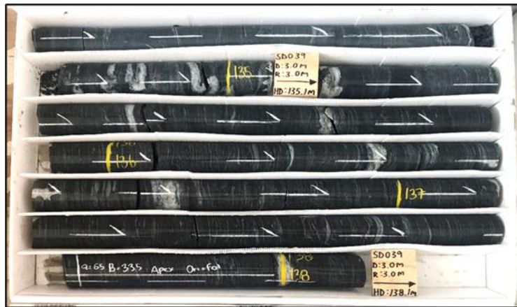
Figure 10-9: SD039, box #36, 134.2–138.1 m, displaying marked up core with orientation marks.
