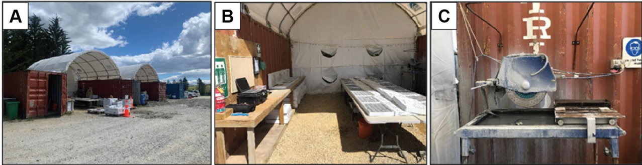
Figure 11-1: A) core storage and logging facility at the Smylers Gold Project; B) core logging set up; C) core saw.
