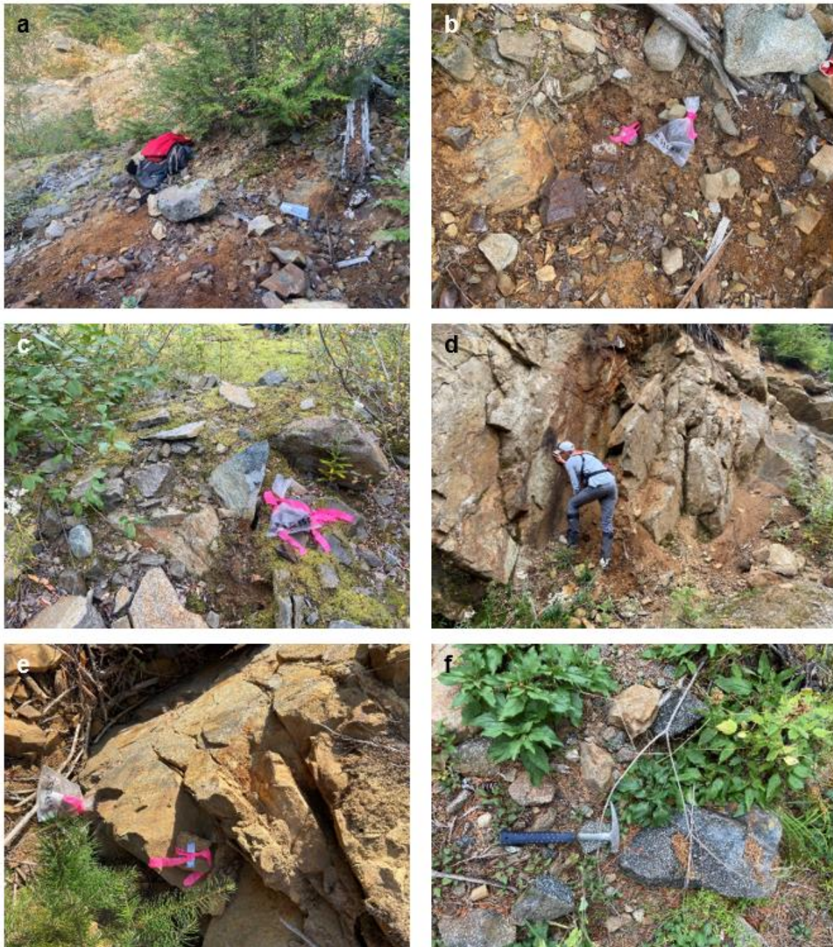
Figure 12-1: Photos taken as part of the QP site visit on 26 September 2022 including (a, b) the massive sulphide boulder comprising the Big Nic showing that is now mostly obliterated through sampling and occurs mostly with monzodiorite boulders (R532854), (c) massive sulphide boulder from an anthropogenically transported boulder pile (R532855), (d) sulphide mineralization on the northeast side of a metapelite xenolith within monzodiorite at American Creek West (R532857), (e) pyroxenite outcrop at the Swede showing (R532859), and (f) feldspathic hornblendite just west of the Swede showing (Source: Equity, 2022).
