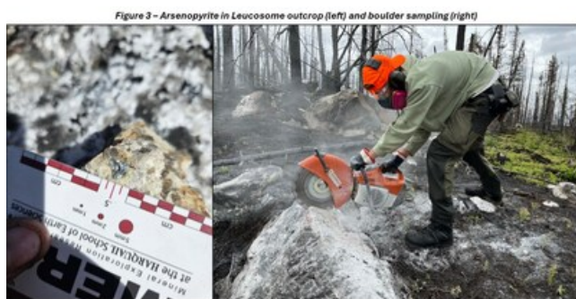
Figure 3 - Arsenopyrite in leucosome outcrop (left) and boulder sampling (right) (CNW Group/Targa Exploration Corp.)
