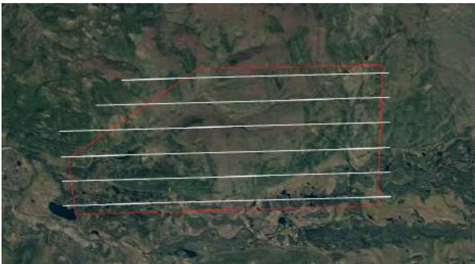
Figure 9.1 Shanghai Property (red outline) with LiDAR Survey Flight lines (white).
