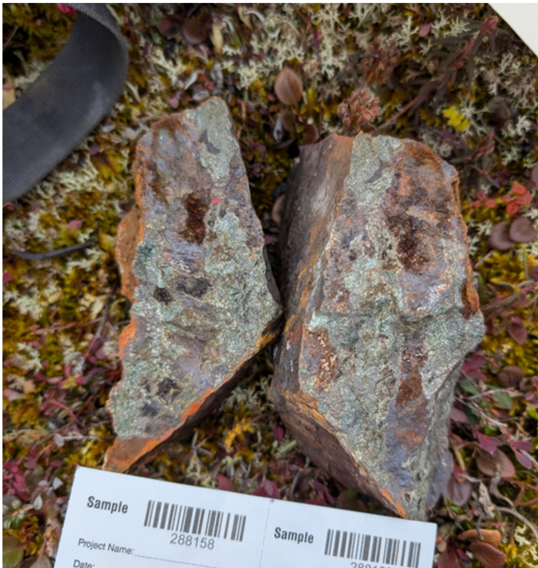
Figure 7- Rock Sample 288158 of mineralized skarn grading 2.42% Cu, 0.94 g/t Au and 42.1 g/t Ag
