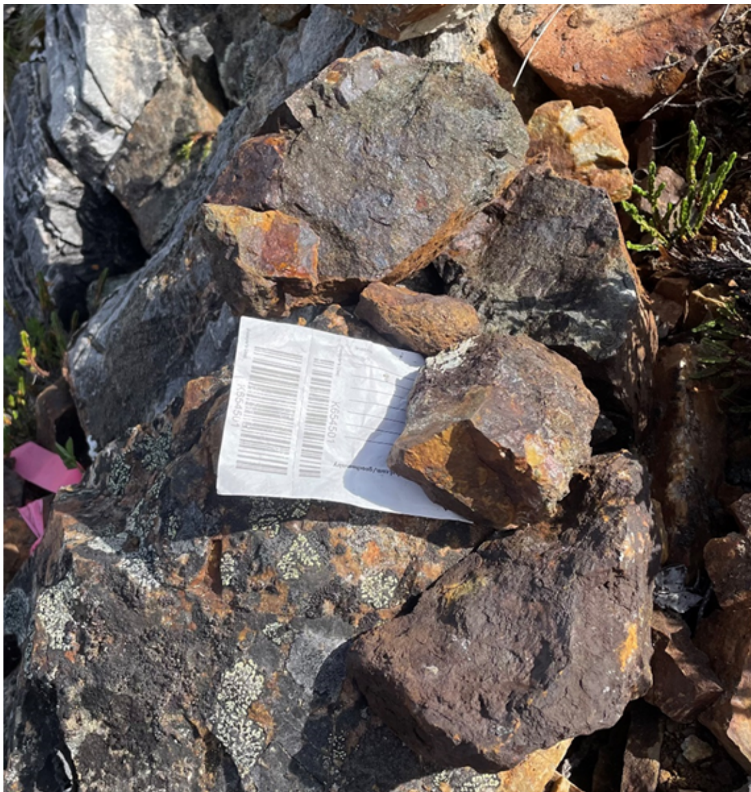
Figure 5- Rock Sample K654501 of mineralized skarn horizon grading 14.1 g/t Au and 4,260 ppm Cu.
