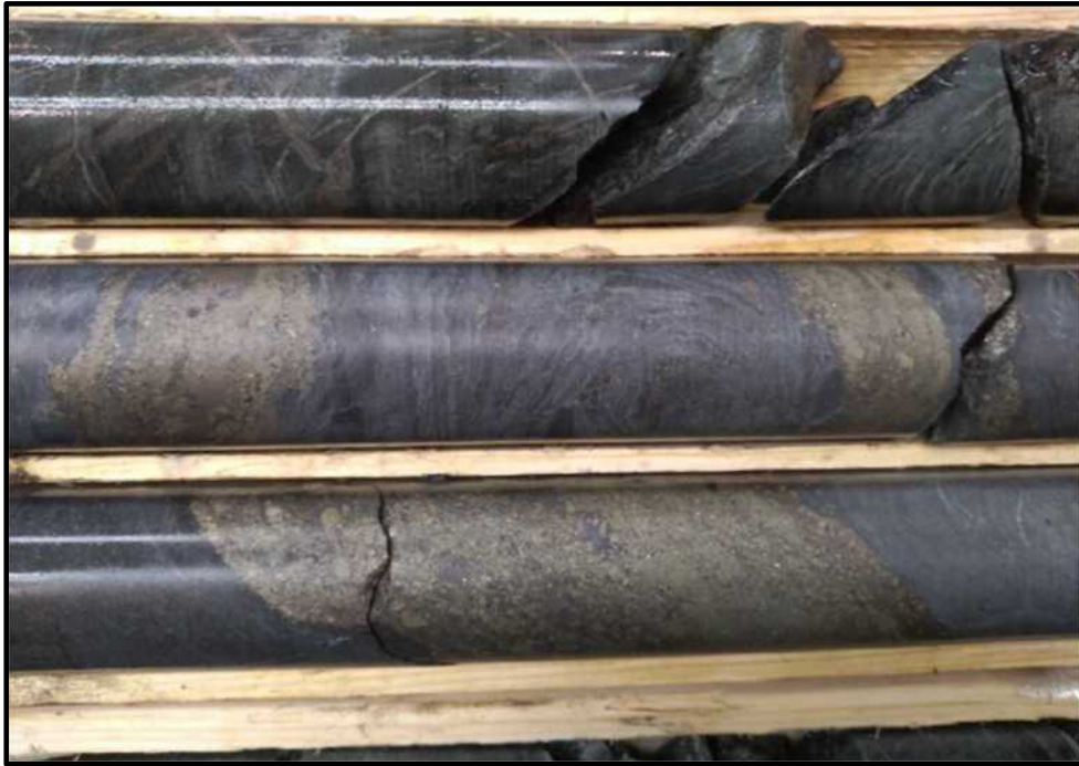
Figure 10 – Sulphide-rich zone in Miniac property drill core
