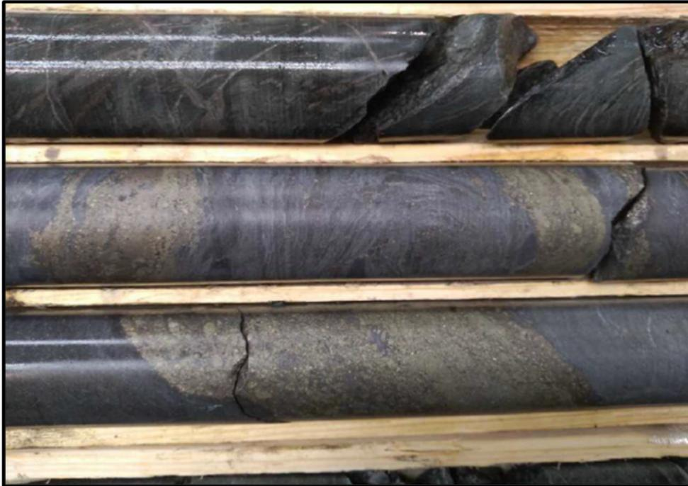
**Figure 10** – Sulphide-rich zone in Miniac property drill core
