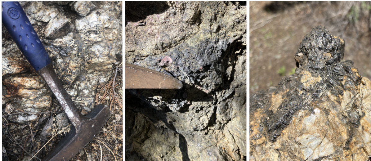
Figure 24. Graphite in fractures (left), graphite seam near Ground Hog (middle), clotty graphite with pegmatite (right).
