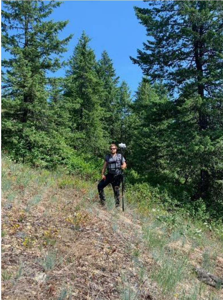
Photo 5: Mag-VLF Survey in progress
