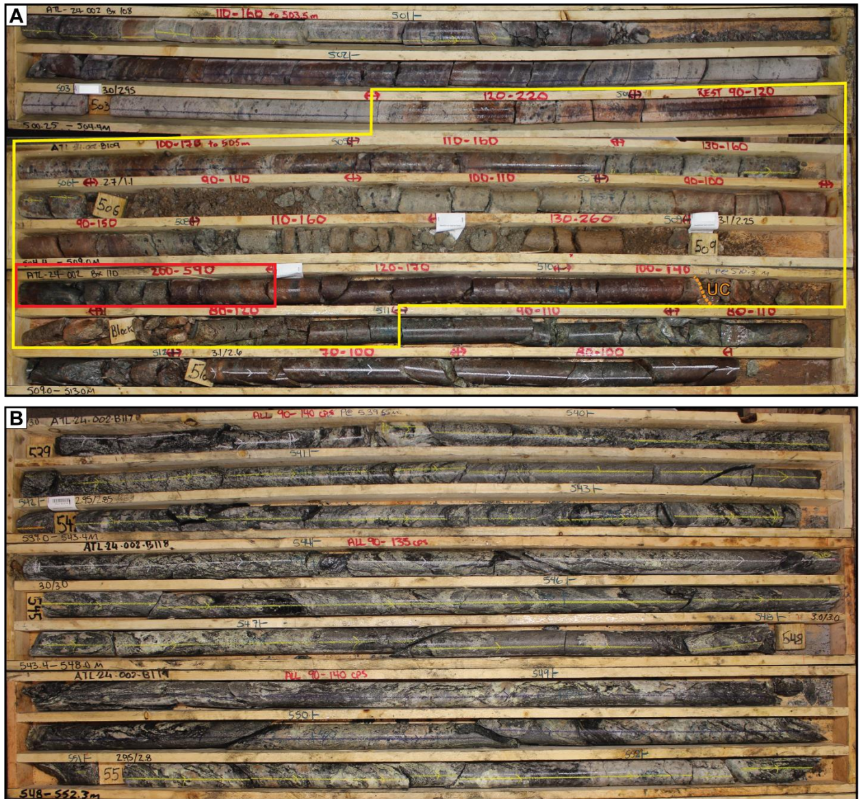
Figure 3. Core photos from drill hole ATL-24-002 highlighting significant structure and alteration intersected in the Athabasca sandstone and basement rocks. UC = Unconformity. A) Variably altered Athabasca sandstone throughout a highly structured interval above the unconformity (yellow box) hosting local anomalous radioactivity (red box) and dravite alteration at the UC. Maximum gamma probe reading of 1,204 cps at 506.3 m. B) Strongly deformed graphitic basement rocks displaying reactivation textures and variable alteration; 539 to 552.3 m.
