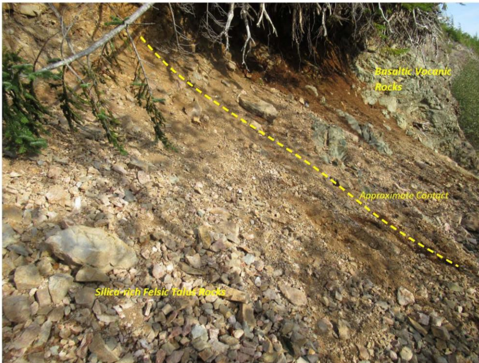
Photo 6 Shows northeastern section of road cut showing basaltic volcanic rock outcrop in approximate contact with silica-rich talus. Dominant talus material consists of thinly laminated silica-potassic layering.
