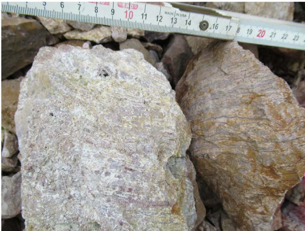
Photo 6 Shows northeastern section of road cut showing basaltic volcanic rock outcrop in approximate contact with silica-rich talus. Dominant talus material consists of thinly laminated silica-potassic layering.
