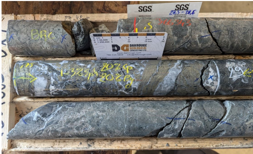
Figure 4: Semi-massive chalcopyrite and pyrite with trace sphalerite mineralization associated with quartz-carbonate veining from 28.75-29.05m in VB24-003.
