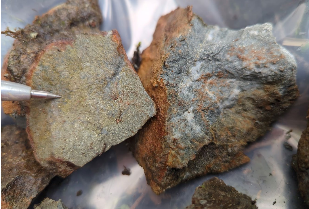
Figure 2: Strongly silicified and sulphide rich samples east of Gregory River in the Jumbo-Lode claim block
