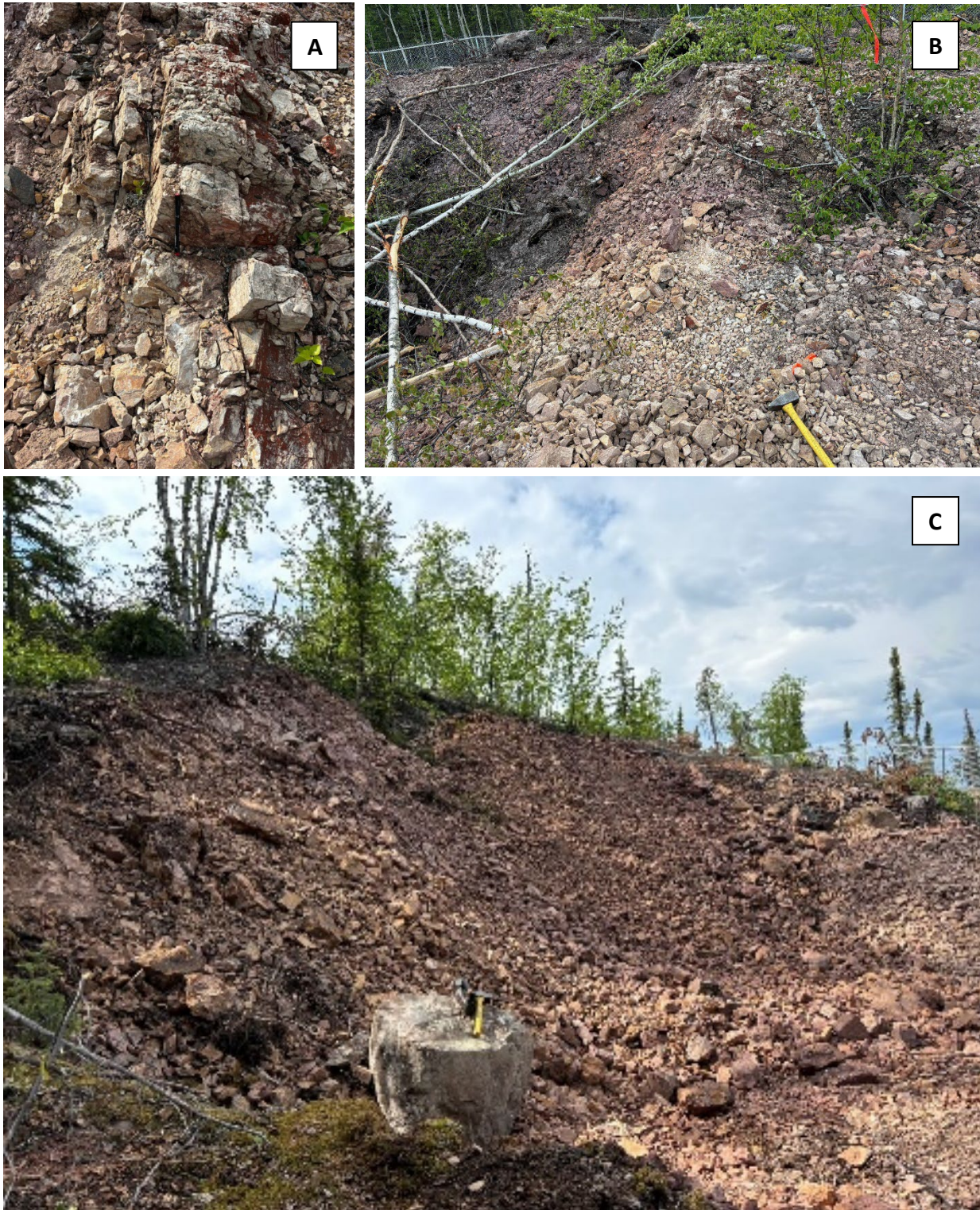
Figure 12.1.8. A) and B) Historic Black Bay Uranium Mine with yellow secondary U mineralization in quartzite fractured along 120°/045° with 0.456% U and 288 ppm Th; C) A blast pit in pinkish quartzites.
