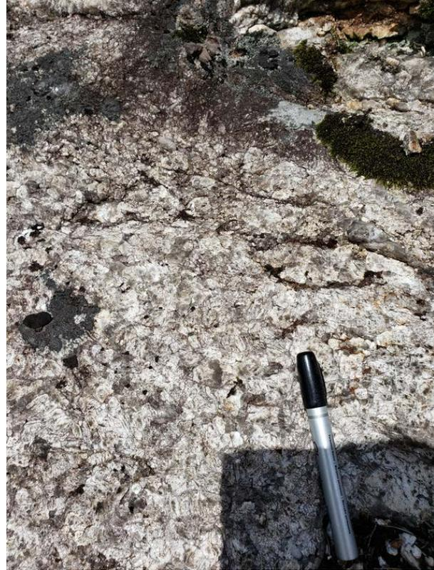
**Figure 12-2: Pegmatitic coarse grained, massive, quartz + feldspar, sampled material for sample Upin2\_JPL22 (Table 12-1).**
