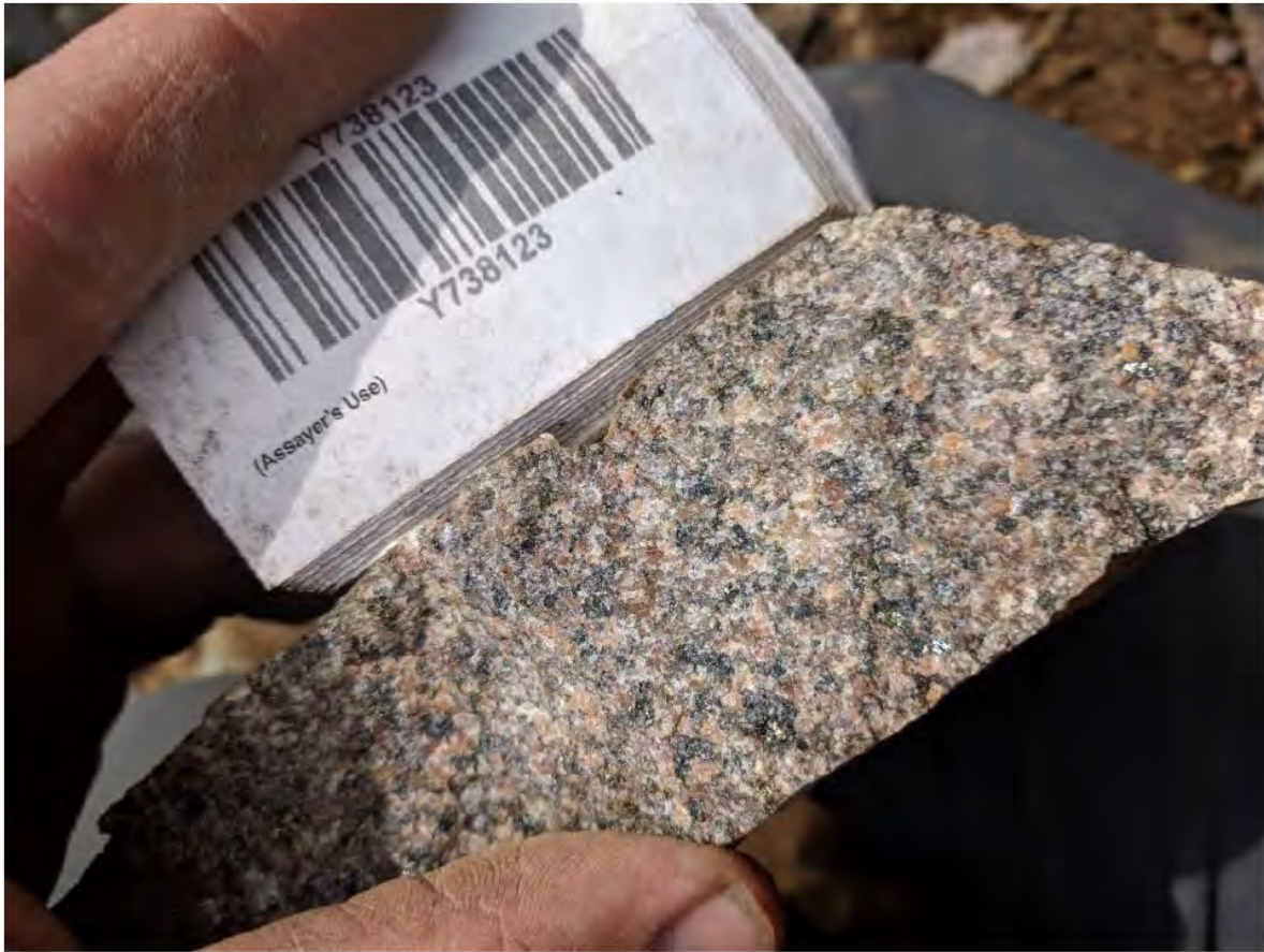
Figure 13. 2019 photo showing mineralized granodiorite at the Loljuh Project showing; 1553 ppm Cu, 11 ppb Au and 1.6 ppm Ag (Michell, 2019)
