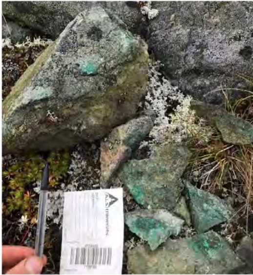
Figure 20. 2019 photo of the skarn at the Chalcopyrite-Bornite Zone; 1.44% Cu, 6 ppb Au and 12.2 g/t Ag. (Michell, 2019)
