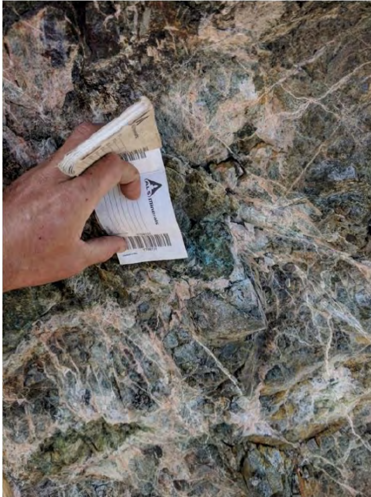
Figure 17. 2019 photo of stock work veins at the skarn and stockwork zone; 0.47% Cu, 659 ppb Au and 5.1 g/t Ag. (Michell, 2019)
