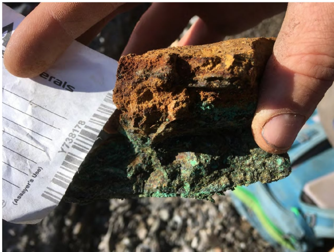
Figure 16. 2019 photo showing grab of mineralized brittle shear zone at Pete Showing; 4.28% Cu, 277 ppb Au and 31.9 g/t Ag. (Michell, 2019)
