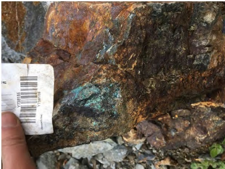
Figure 19. 2019 photo of the Magnetite-Chalcopyrite Vein occurrence; semi-massive magnetite vein; 5.00% Cu, 1.177 g/t Au and 30.7 g/t Ag. (Michell, 2019)
