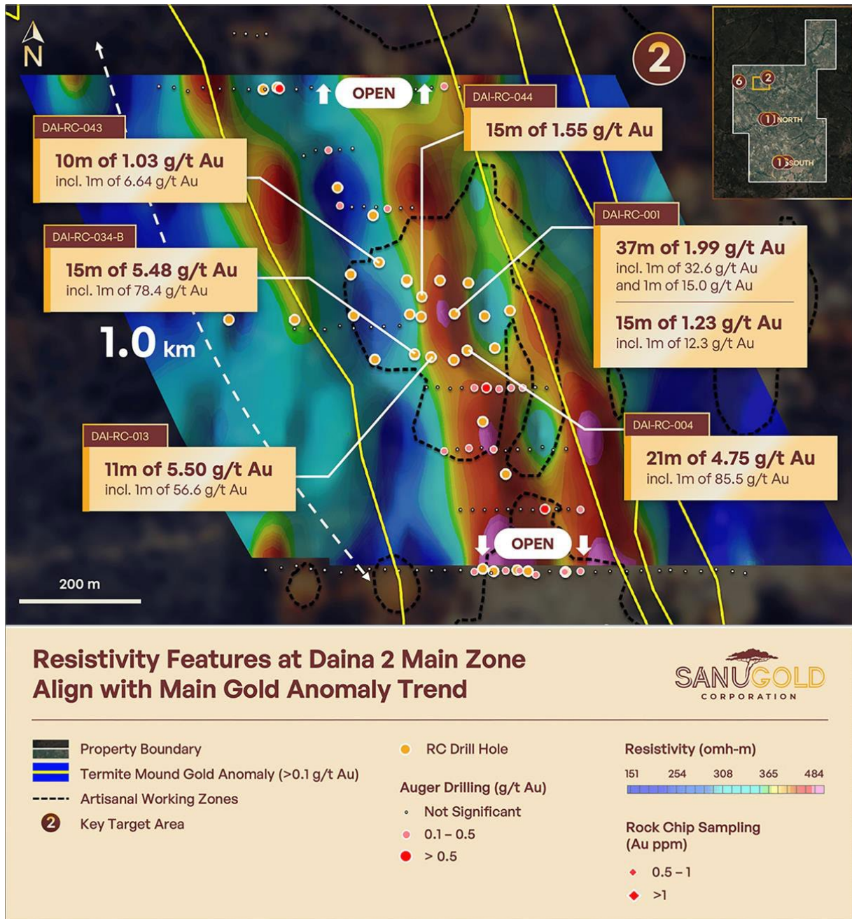
Figure 4: Daina 2 Target, surface geochemistry gold anomalies and gold in saprolite anomalous points from auger drilling over ground geophysics image (Chargeability).
