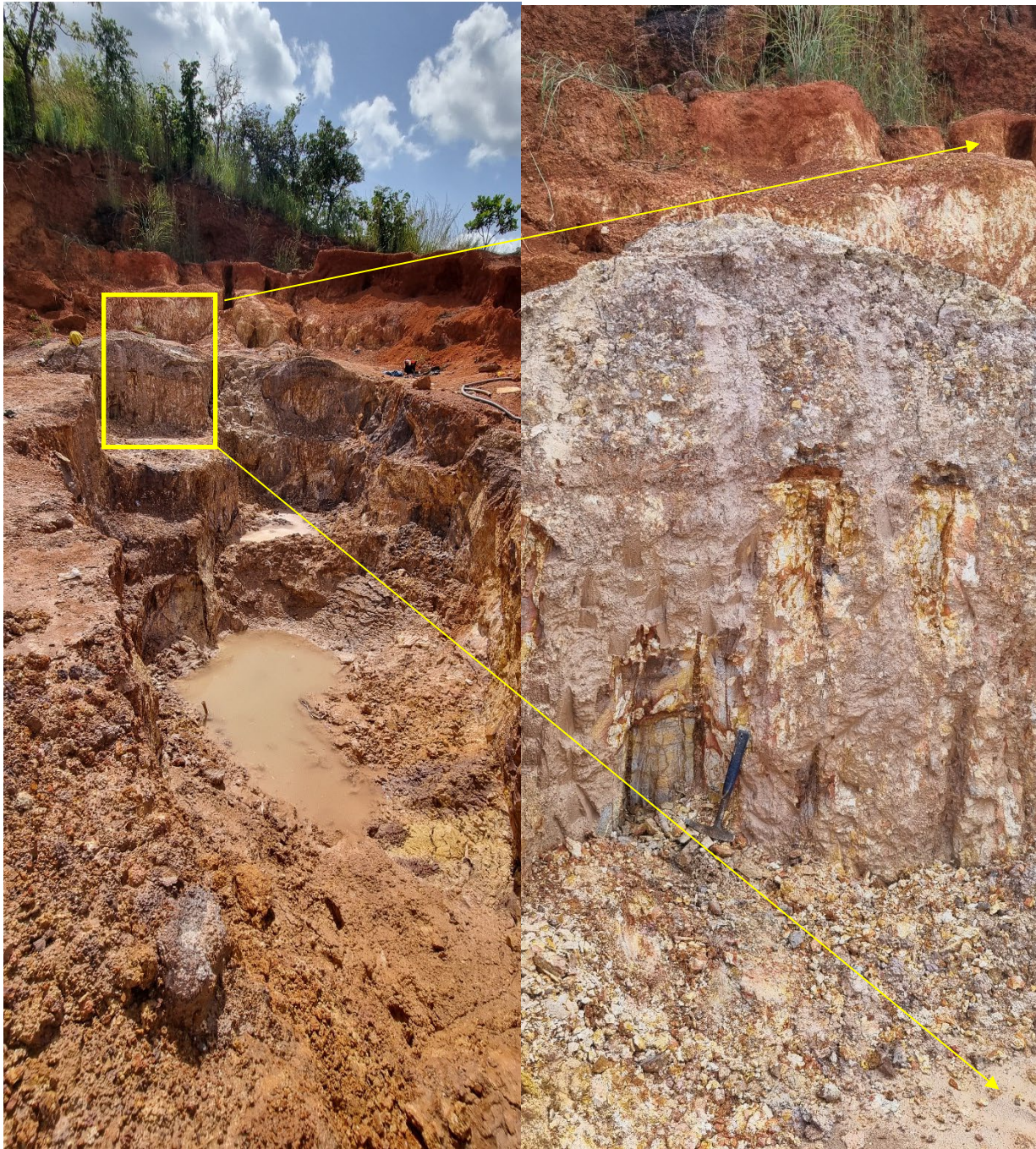
Photo 2: Workings exploiting altered and quartz veined greywacke units with subvertical, north east trending veinlets.
