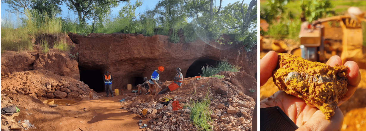
Photo 3: Entrance to active artisanal underground workings, inset shows material mined, sediments weathered to saprolite with dark grey quartz veinlets.
