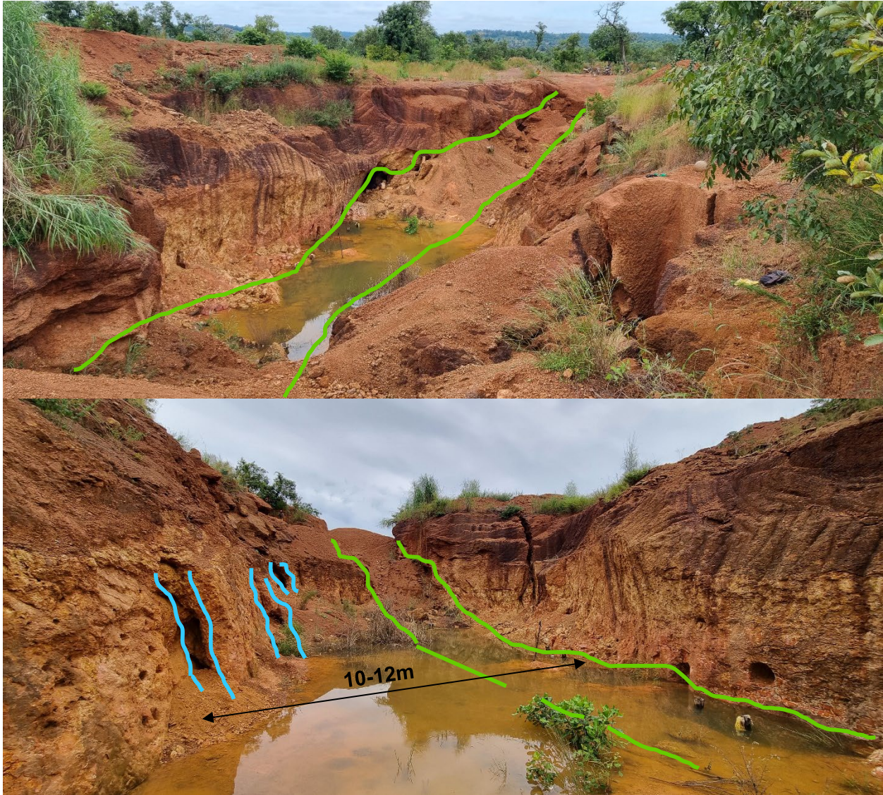
Figure 3: Workings at Salat East in the weathered granite, exploiting a 70 degree west dipping structure 5-8m in width. Upper photo view along strike to the northeast. Lower Photo: View along strike to the southwest. Green lined denote limits of main exploited structure. Blue lines show sub parallel footwall structures exploited.
