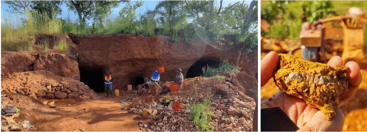
Photo 1: Entrance to active artisanal underground workings, inset shows material mined, sediments weathered to saprolite with dark grey quartz veinlets.
