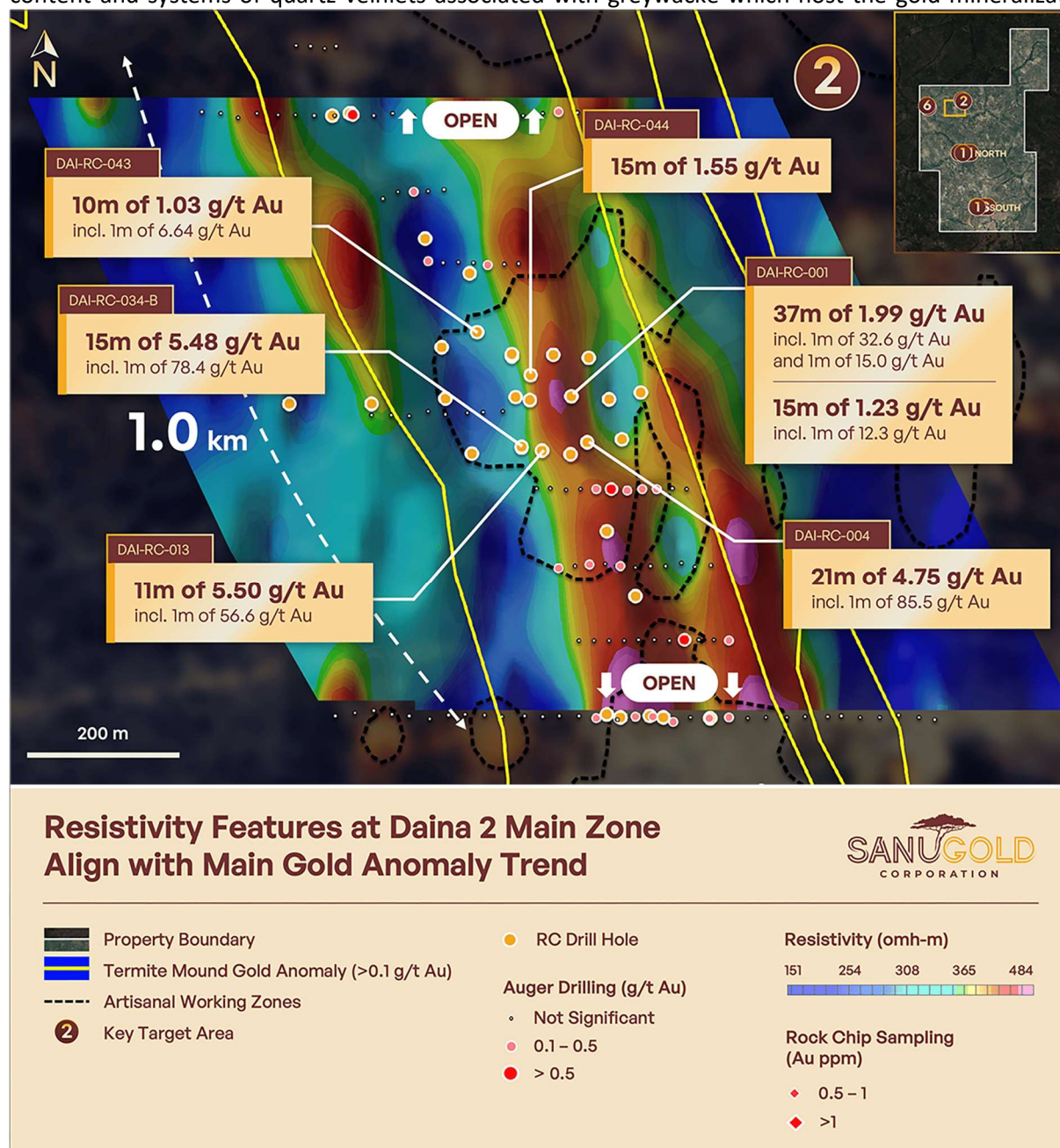
Figure 4: Resistivity features at Daina 2, previous RC drill location with intercept highlights, auger samples, termite gold anomalies, extend of artisanal surface workings and planned extensions to the IP surveys.
