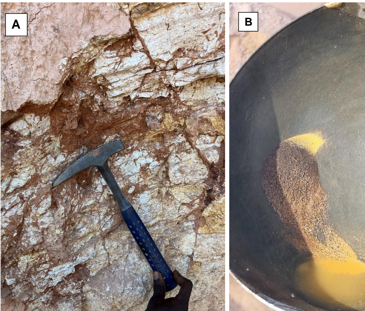
Figure 5: Target 7 mineralization: A) outcrop of oxidized felsic intrusive with quartz veining and boxwork after sulphide; B) free gold panned from surface workings.
