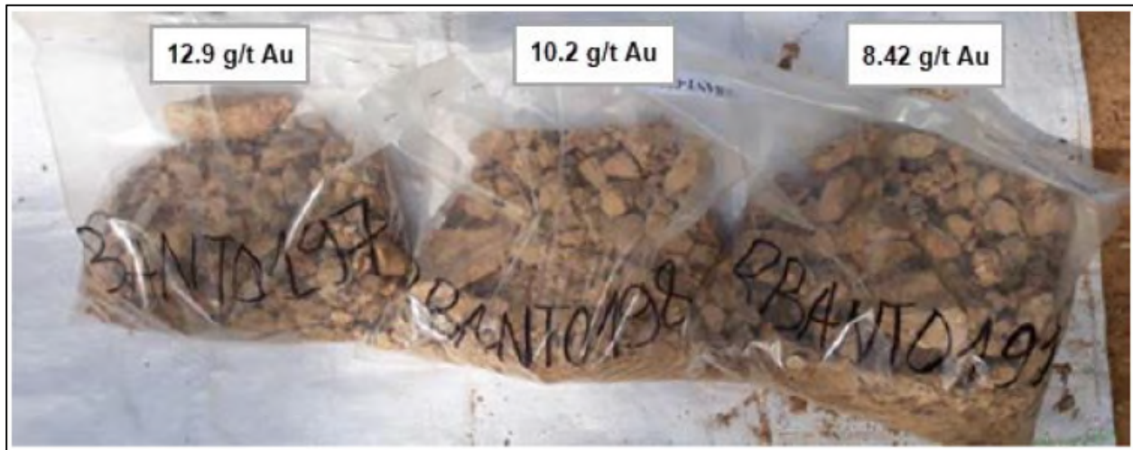
Figure 25 - Samples of Altered Volcanoclastic Rocks that Returned Significant Results for Au from Pit Samples
