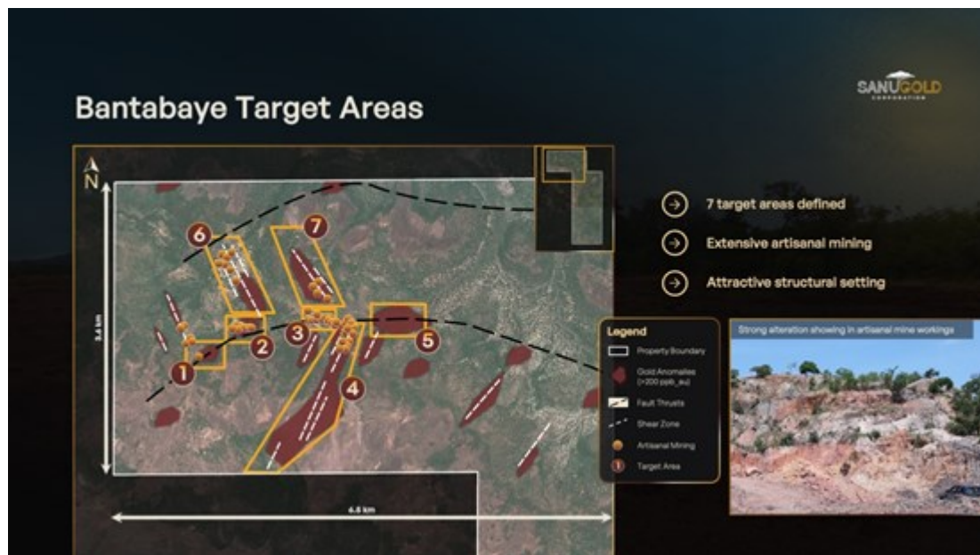
Figure 4: Bantabaye Permit, gold anomalies defined from historic termite mound geochemistry, structural trends and occurrences of artisanal workings
