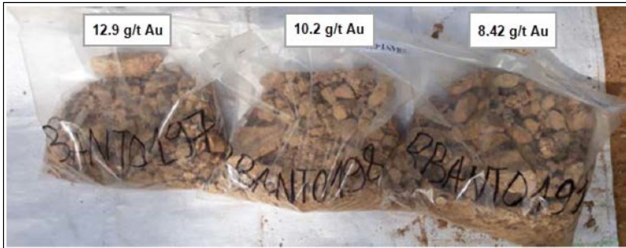
Figure 24 - Samples of Altered Volcanoclastic Rocks that Returned Significant Results for Au from Pit Samples
