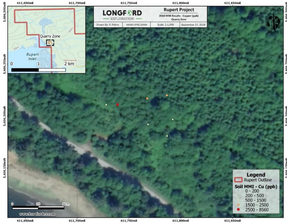
Figure 6-2 MMI Sample Locations in the Northwest (quarry area) with colour coding copper value ranges
