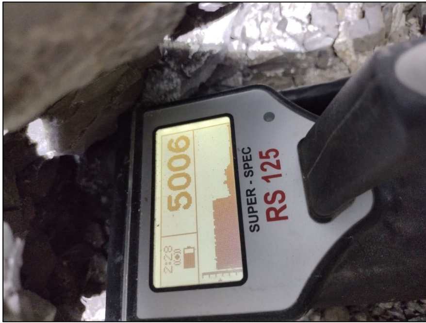
Figure 3 – Scintillometer reading of 5,000 cps at assay location
