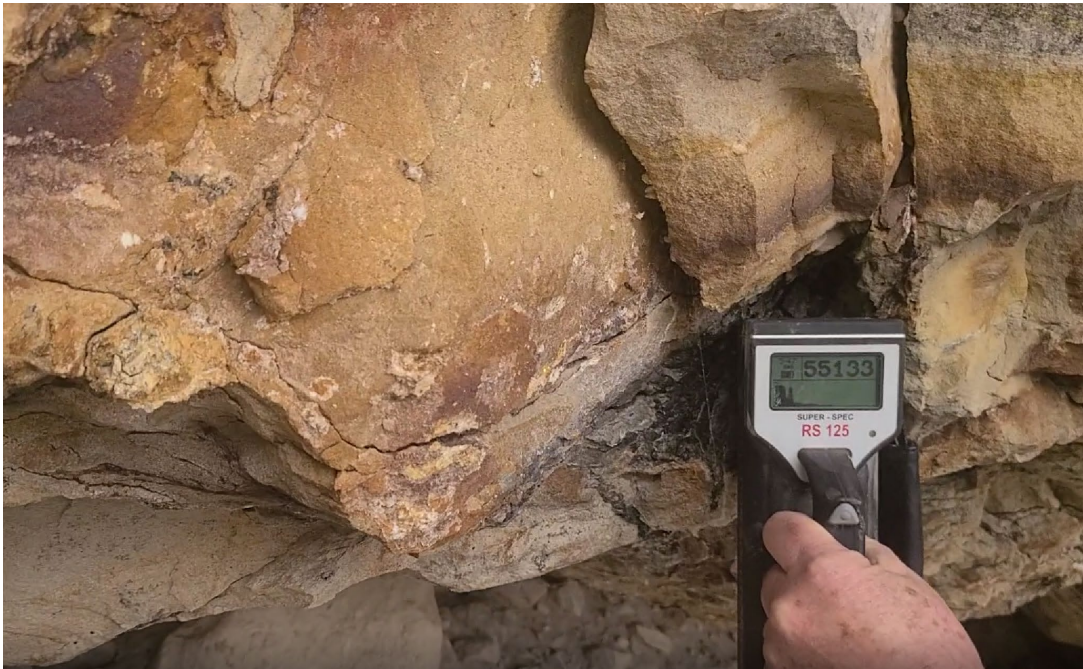
Figure 5 – George measuring over 55,000 cps near the Acerson historical workings.
