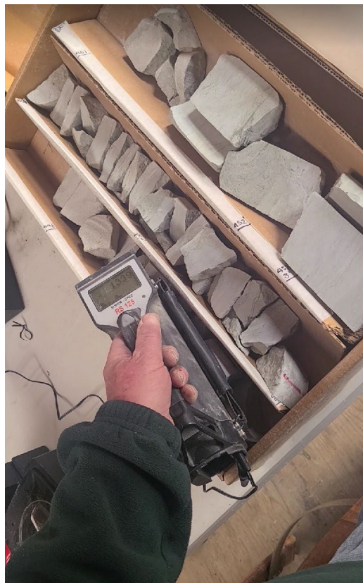
Figure 1 - GR-1003 reading elevated gamma counts of over 1,300 cps at ~ 448.5 ft . 2006 assays state average of 0.10% eU3O8 between 446.5 and 449.0 ft (historical)
