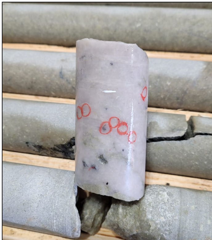
Figure 1. TL-23-001 core, 11 separate flecks of visible gold were recorded by geologists.
